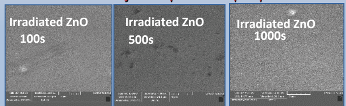
Surface morphology of thin films exposed to 3 MeV alpha radion.
